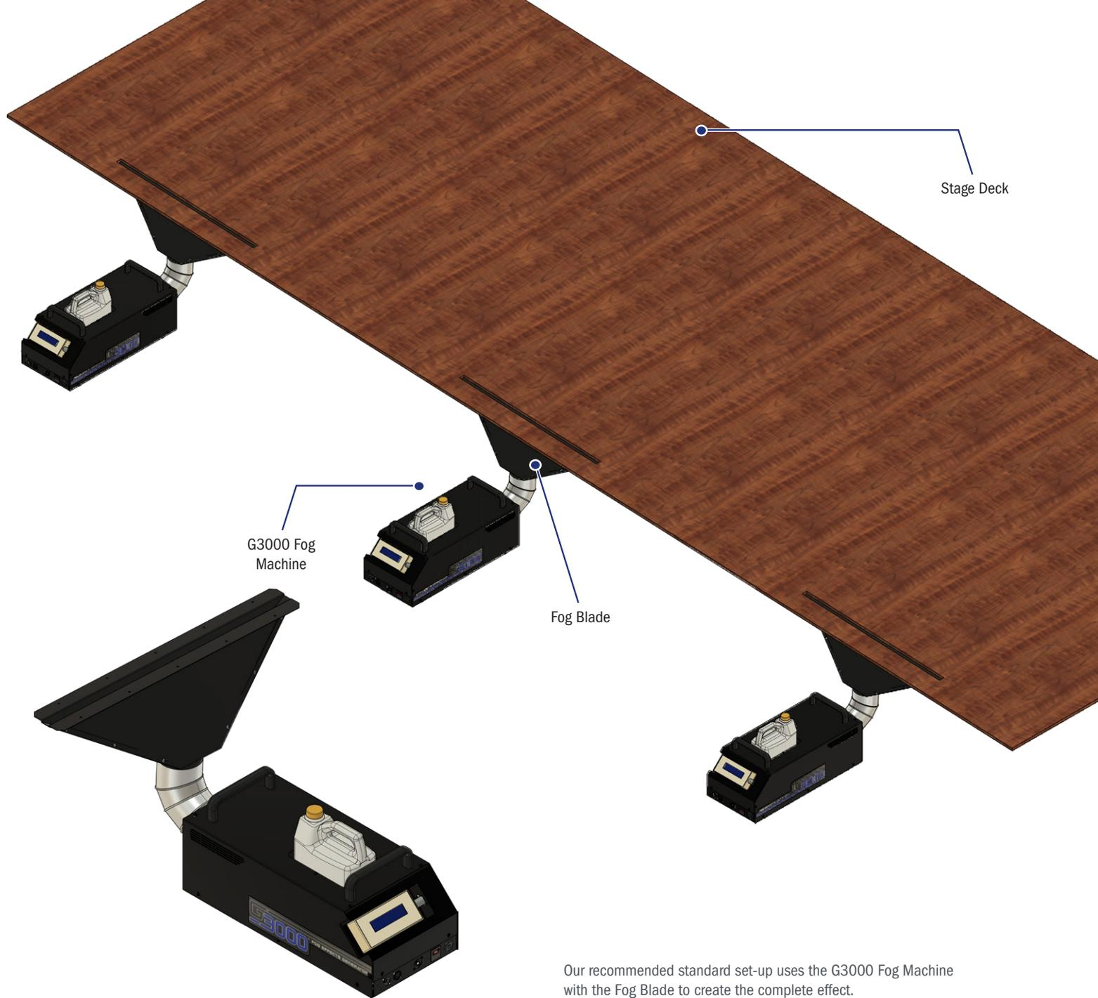
Our recommended standard set-up uses the G3000 Fog Machine with the Fog Blade to create the complete effect.
